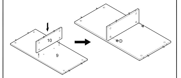
Attach panel (10) to panel (9) using cam bolts and dowels as guides. Secure panel (10) to panel (9) using cam locks (D). Tighten cam locks (D) with a screwdriver.
